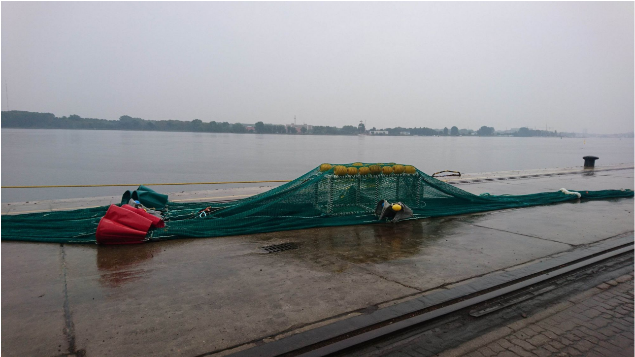
Figure 7: Lateral view of the experimental FD40_110 codend surrounded by the cover. The cover was rigged with forward (red, green and grey) and lateral kites aligned to the mid-length of the codend (grey). To compensate for the negative buoyancy of the FD40_110 codend, the device was initially rigged with 2x floating lines consisting of 7x foam buoys that were attached side by side along the longitudinal upper bars of the frame.
