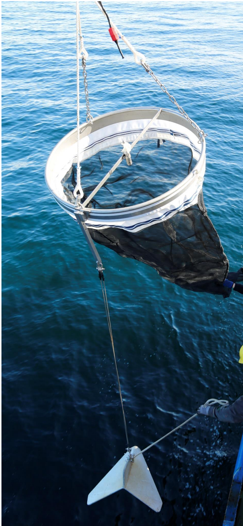
Figure 8: CalCOFI-plankton-trawl in configuration 1 (see Table 1) during deployment (note, the attachment of the depressor to a lever arm and equal length of bridles)
