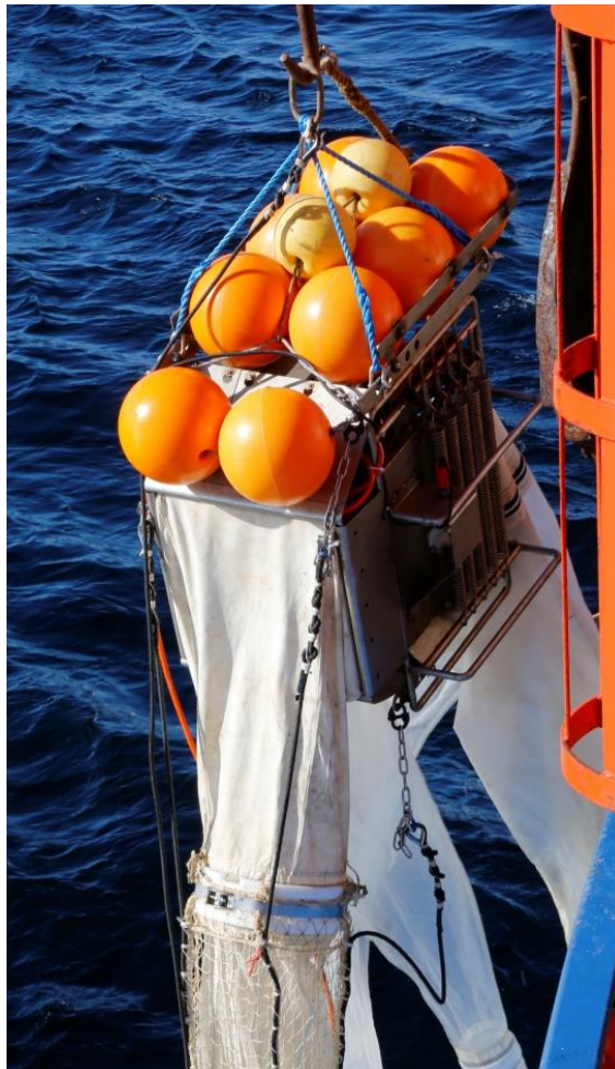
Figure 6: Hydrobios-Multisampler (size midi, 0,25m 2 ), attached to the aftend of the IKMT
